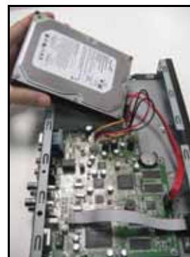
Figure 27.3 Carefully remove the HDD from housing.
